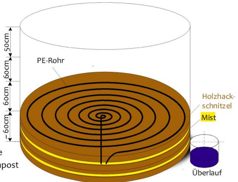
Put in two more spirals at a height of 70 cm. After the third spiral 80 cms worth of material should be added. This layer will not heat that much. It serves primarily as an insulator and protects the Eco-Kiln. Additionally, in this third and last layer of material, there will be aerobic processes that are reliant on the anaerobic surface processes.
